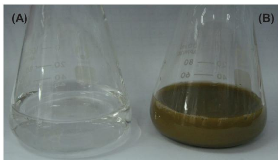
Figure 2 Aqueous solution of 10^{-3} M \text{AgNO}_3 with pu-erh tea leaves extract (A) before adding the tea extract and (B)
